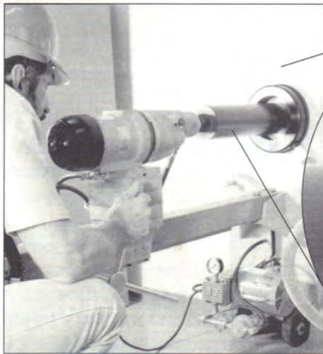
A typical SLURRY SLURP installation on a coring drill using a standard shop vacuum.
